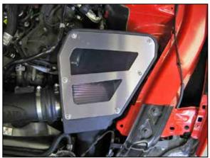
21. Install the clear and aluminum lids onto the air filter housing and secure with the provided hardware.
