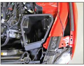
15. Install the AIRAID® air filter assembly into the vehicle and secure with the provided hardware.
