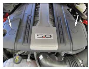
3. Remove the two covers to access the nuts that secure the engine cover, then remove the two nuts and engine cover.
