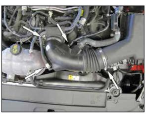
5. Disconnect the two vent lines attached to the factory intake tube, loosen the hose clamps that secure the intake tube to the throttle body and air filter housing.
