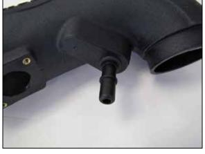
12. Install the large quick disconnect fitting into the AIRAID® intake tube using the provided grommet.
